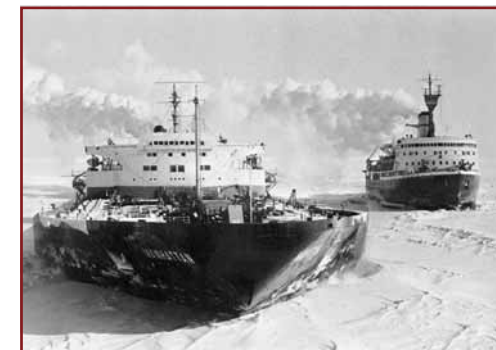
Lukens steel went into the S.S. Manhattan, the first commercial vessel to transit the "Top of the World" route.
